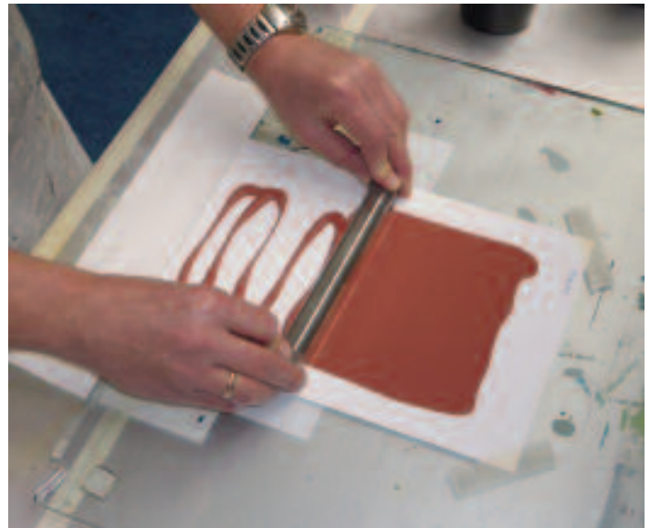
Drawdown bar is used to create film of uniform density prior to color evaluation.
