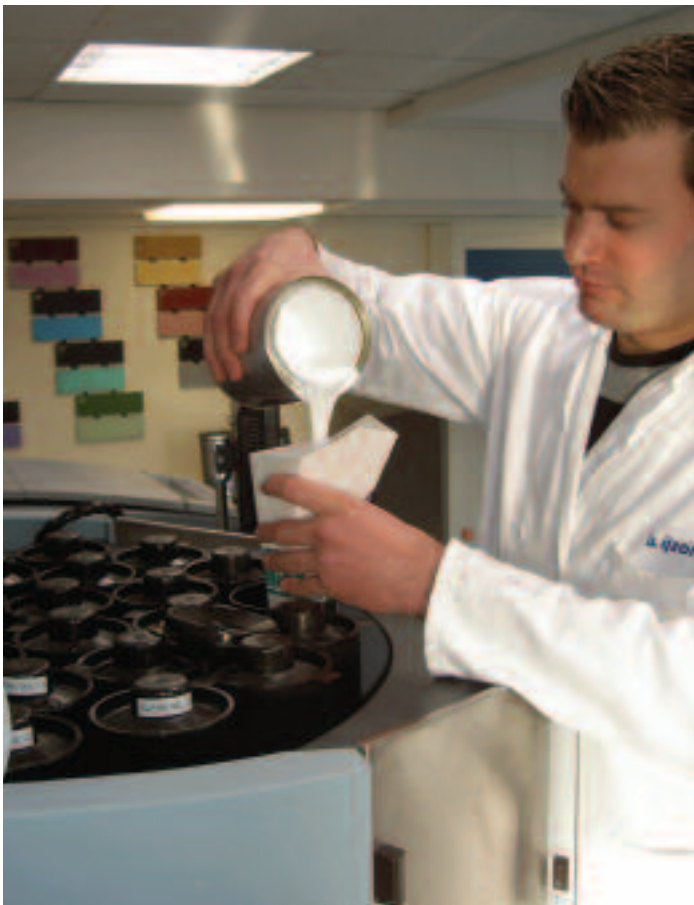
Colorants are loaded in dispenser with paper funnel, that's certainly not a filter.
